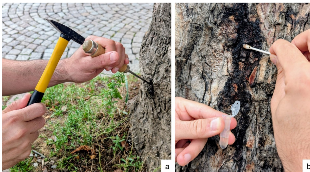
Fig. 2 Sampling methods a : sampling with hammer and chisel; b : sampling with cotton swab
